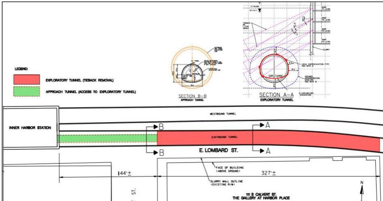
**Figure 8: Concept of SEM Tunnel for Tieback Removal**
