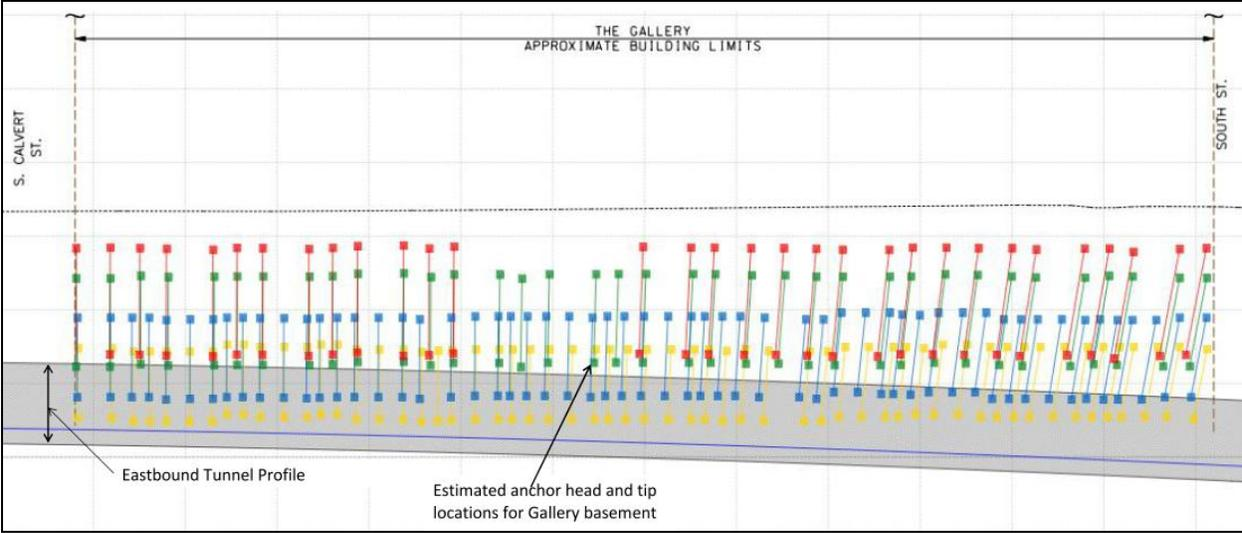
**Figure 5: Tunnel Profile with Estimated Anchor Obstructions**
