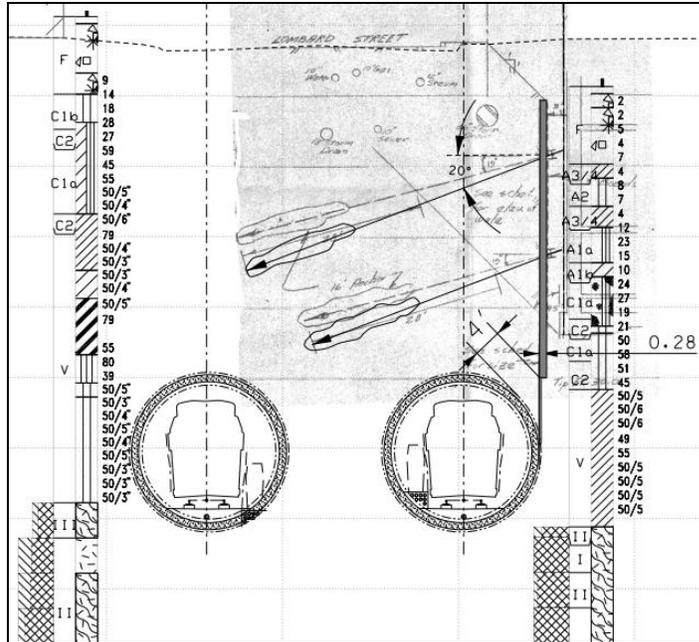
**Figure 3: Estimated Proximity of Soldier Piles and Tiebacks to TBM tunnels, West Approach to Inner Harbor Station**
