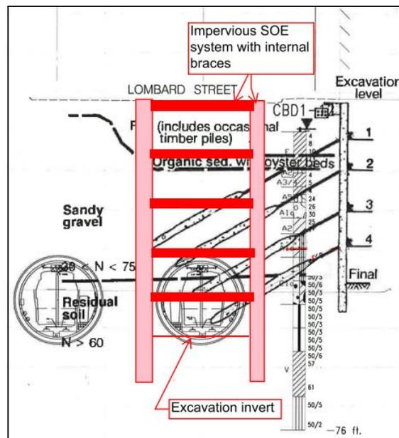
**Figure 6: Concept of Cut-and-Cover Excavation for Tieback Removal**
