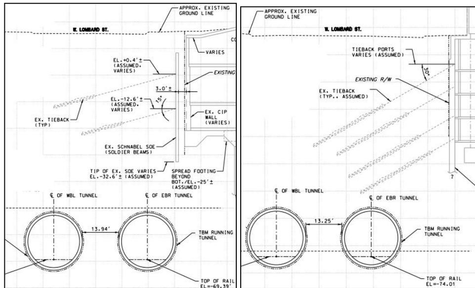
**Figure 9: Sections at TransAmerica and Gallery Buildings for Three Level Inner Harbor Station Alignment**
