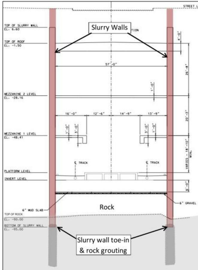
Figure 5: Station section for rock below station subgrade (Fell's Point Station)
