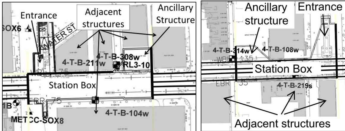
Figure 3. Examples of station layout and proximity of adjacent structures (Inner Harbor and Fell's Point Stations)
