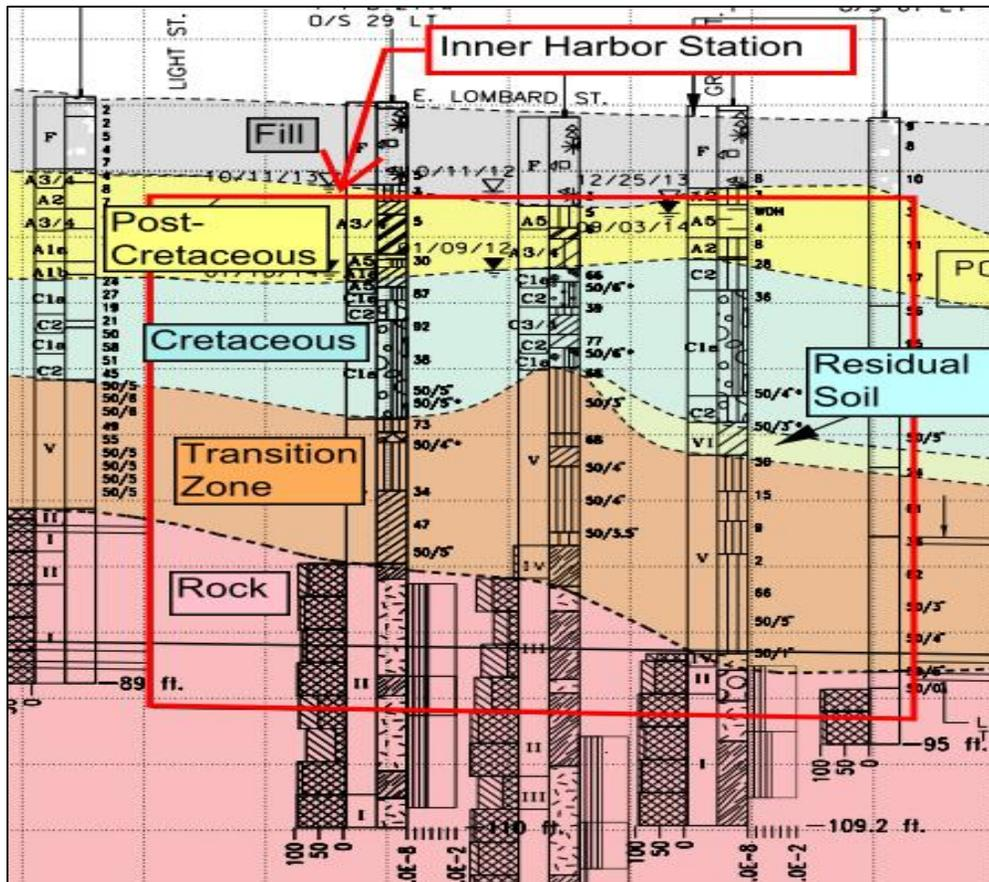
Figure 2. Subsurface profile at Inner Harbor Station
