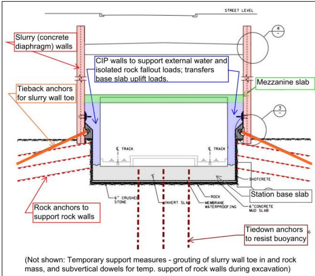
Figure 6: Station design concept for stations within rock (Poppleton Station)
